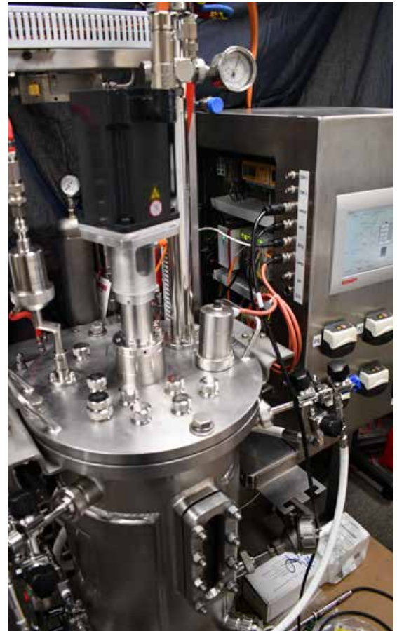
AFC 2000 bioreactor controller designed to work with 40L Sartorius Biostat C reactor
