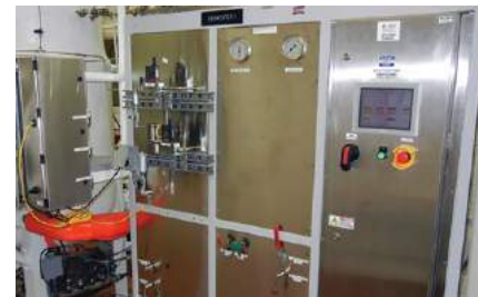
AFC 2000 semi-custom bioreactor controller designed to fit into existing cabinetry
