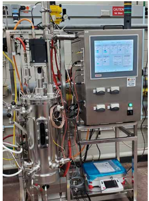
AFC 2000 bioreactor controller designed to work with 40L Sartorius Biostat C reactor
