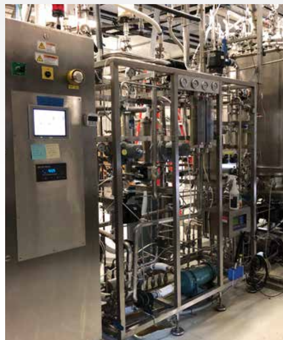
AFC 3000 semi-custom 1500L bioreactor controller
