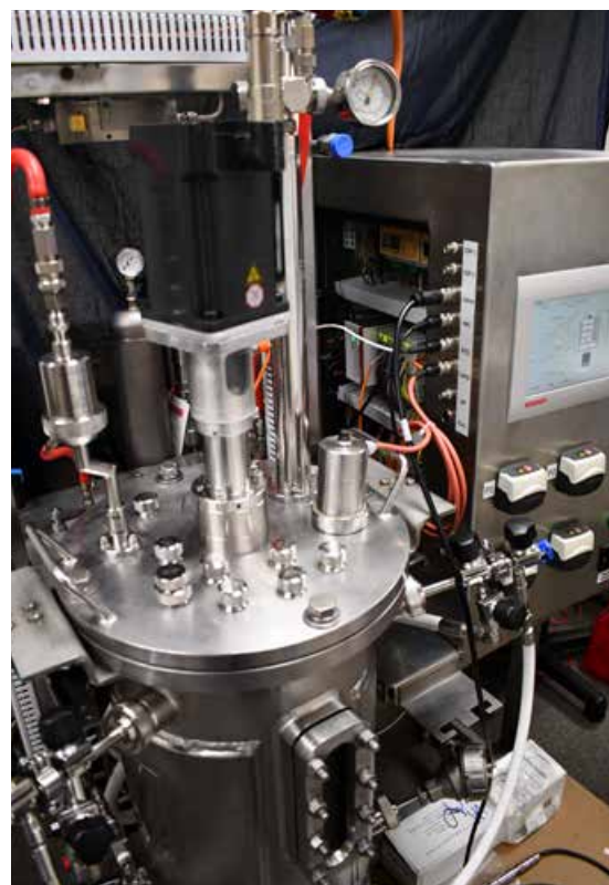
AFC 2000 bioreactor controller designed to work with 40L Sartorius Biostat C reactor
